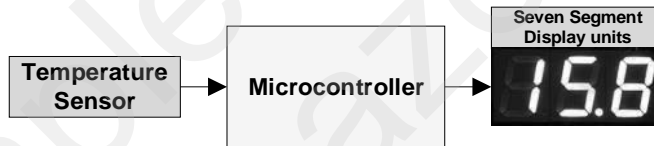
Figure 1.12 Application for displaying temperature using seven segment display units
